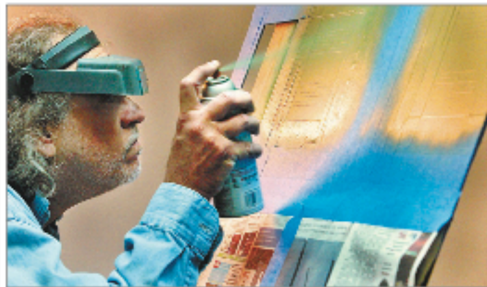
NEW COAT OF PAINT: Model maker Ray Del Papa sprays the first layer of a building mock-up in the paint booth of SMARTT's facilities.
